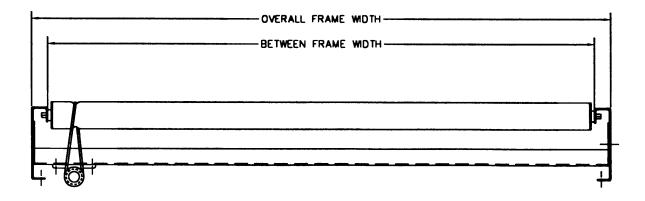
The drive capacity of one roller with a smooth bottom part is 25 pounds maximum. The Standard Bed Length is 10 feet.
