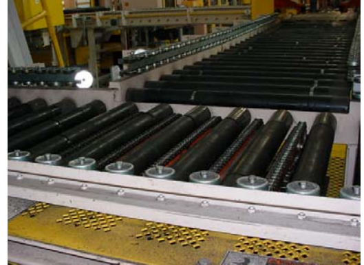
Heavy Duty Five Strand Chain Transfer
