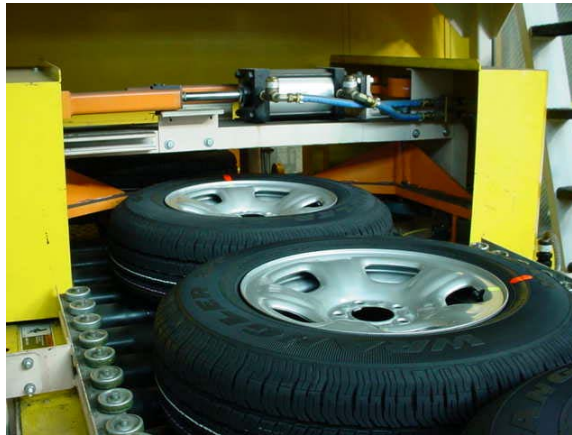
Heavy Duty Five Strand Chain Transfer
